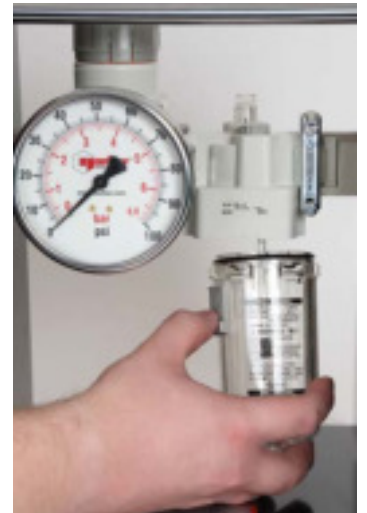
FIGURE 4 – Lubricator Bowl Replacement
